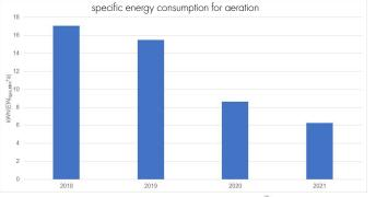
By optimizing the aeration system, energy savings of an extremely impressive 63 % could be achieved, as was shown after the modification in 2021. The investment in highly efficient AEROSTRIP® diffusers has paid off.
